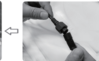
11. Connect the adapter cable between the solar floodlight and the solar panel. Insure that this waterproof connection is secured
