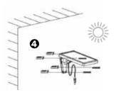
Use the holes on the mounting plate to mark out drill holes. Drill four holes, insert wall plugs and fix the mounting plate with screws. Rotate the solar panel so it is in direct sunlight.
