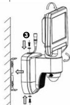
Use two screws to attached the floodlight back onto mounting plate.
